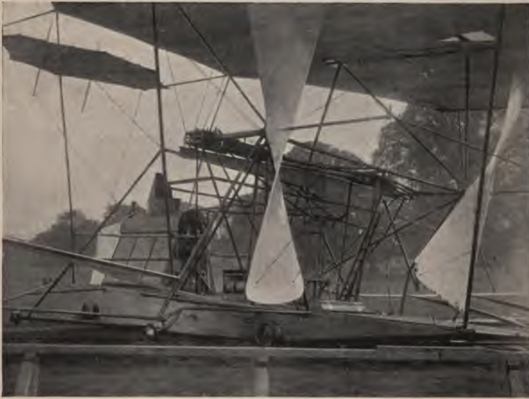
Fig. 83.—This shows the screw damaged by the broken planks; also a hole in the main aeroplane caused by the flying splinters.
